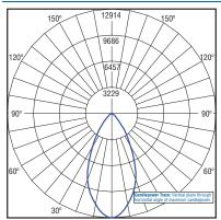
Independent Testing Laboratories certified test. Report No. ITL65015 Candlepower trace of 6000K, 60 LED 40° Flood optic Flood 304 seiries luminaire with 10,625 initial delivered lumens operating at 525mA. All published luminaire photometric testing performed to IESNA LM-79-08 standards.
